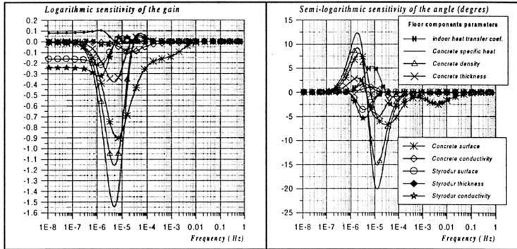
Figure 2: Frequency domain sensitivity to parameters of floor components.
