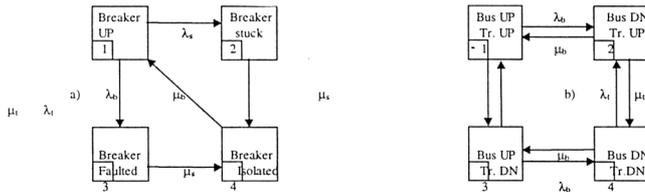
Figure 1: Markov models of circuit breaker (a) and of overlapping failure of bus section and transformers (b)
