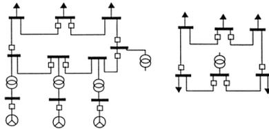
Figure 3: Station configurations: ring bus 13 and 3
