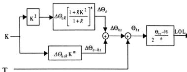
Figure 1 – Block diagram of transformer thermal and loss of life models.
