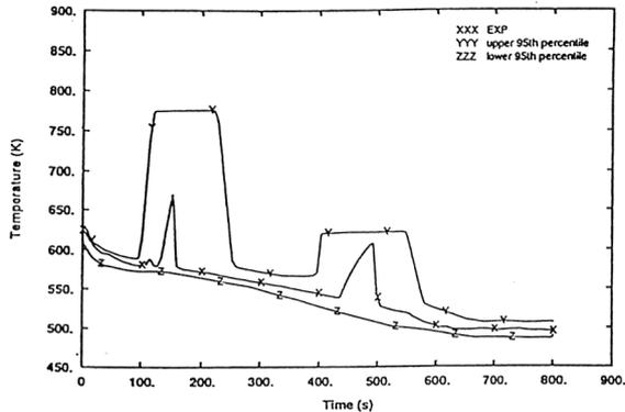
Figure 2: UMS RELAP application : LSTF heater rod temperature (hot rod, pos. 8), nominal calculation result, uncertainty band and experimental trend
