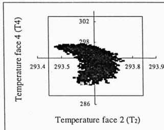
Figure 2 : Comparison between FDDA and MC methods on a highly non-linear convective - radiative thermal exchange model. This figure shows the uncertainties of two temperatures. The solid line gives the uncertainty domain computed with FDDA and the cloud of points gives the results of MC analysis.
