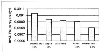
Figure5: Sensitivity of BPSD Frequency on changes of repair and maintenance times
