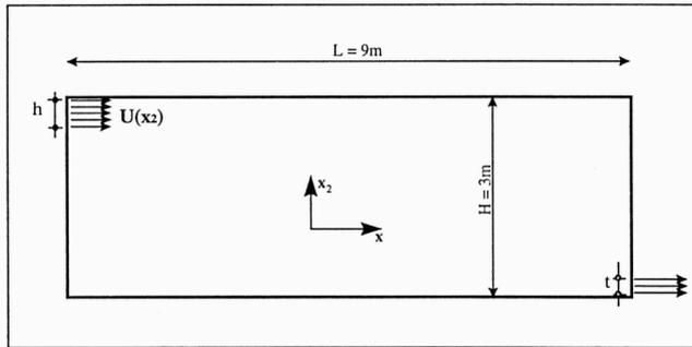
Figure 1: The two-dimensional ventilated enclosure studied.
