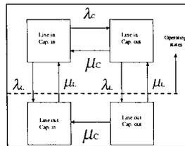
Figure No. 2: State Diagram for a Series Compensated Line
