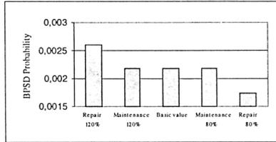
Figure 4: Sensitivity of BPSD Probability on changes of repair and maintenance time
