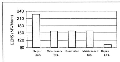
Figure 6: Sensitivity of the EENS on the changes of repair and maintenance times
