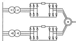
Fig. 1 Twelve pulse electric propulsion scheme
