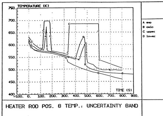
Figure 1: UMS CATHARE application : LSTF heater rod temperature (hot rod, pos. 8), nominal calculation result, uncertainty band and experimental trend
